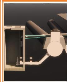
Waste screening keeps out solids from closed loop system
